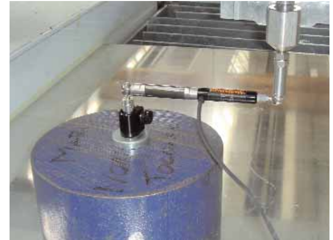
Final "Bench Mark" cutting test
