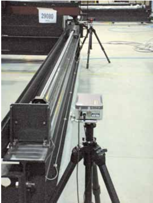
Laser Renishaw for Straightness Control
