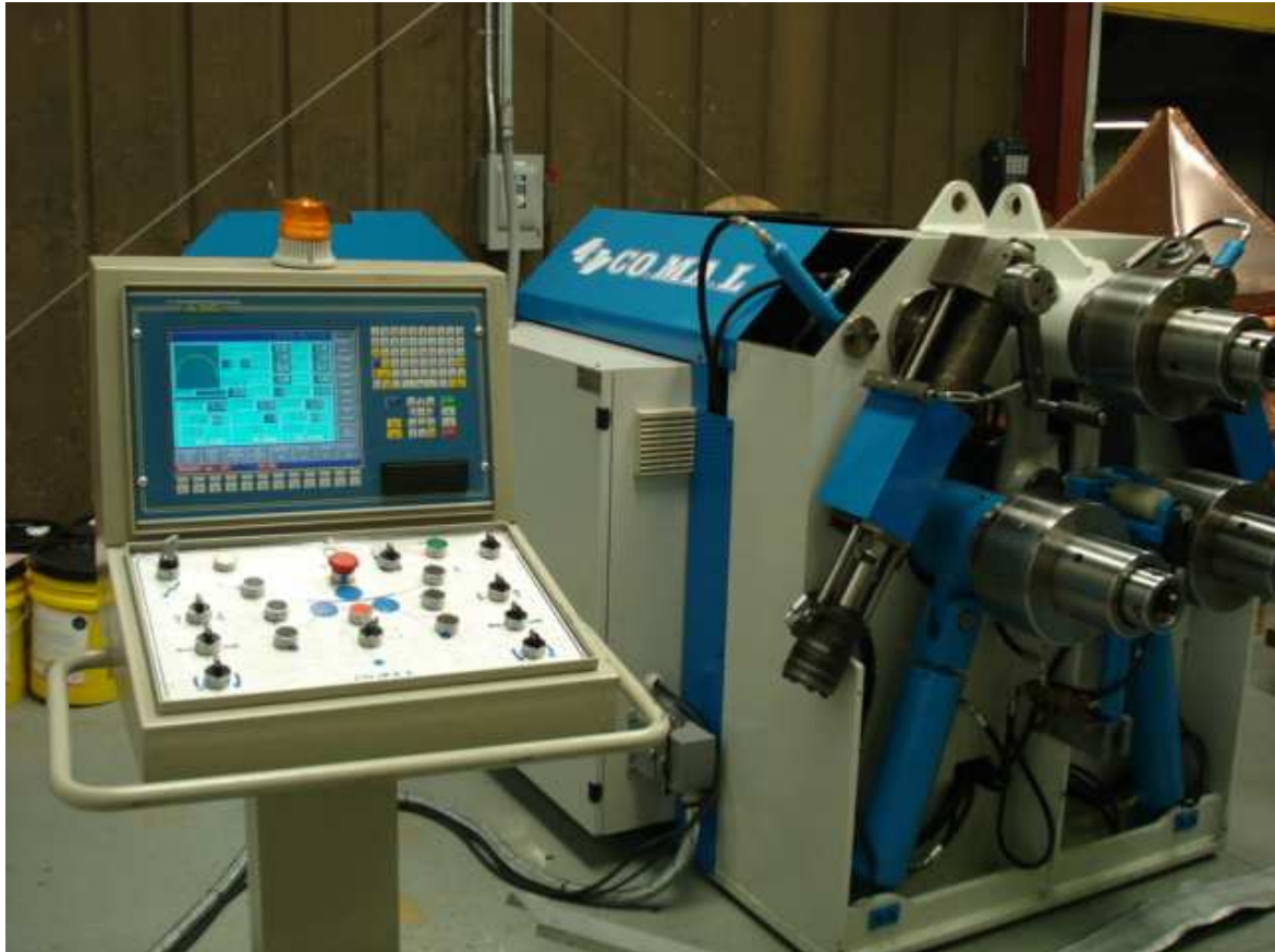
OMEGA 80 with covers removed/ special tooling / hydraulic lateral guides (three degrees of freedom) and the EASY BENDER CNC
